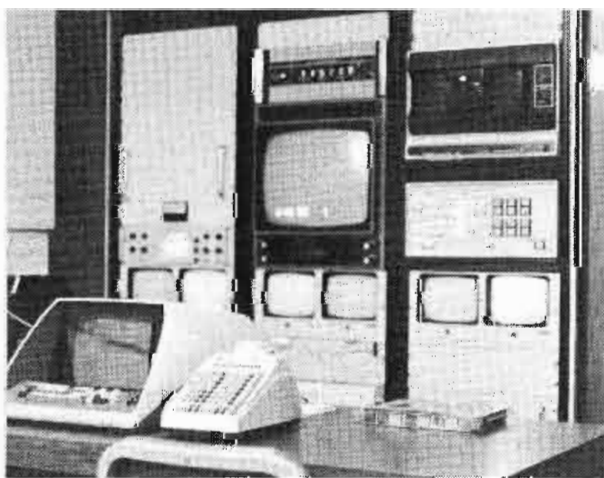
This is the off-line edit bay with CMX computer edit system. After off-line edit on one-inch VTR's, punched paper tape is fed through reader (top right) for auto assembly on two-inch VTR's.
