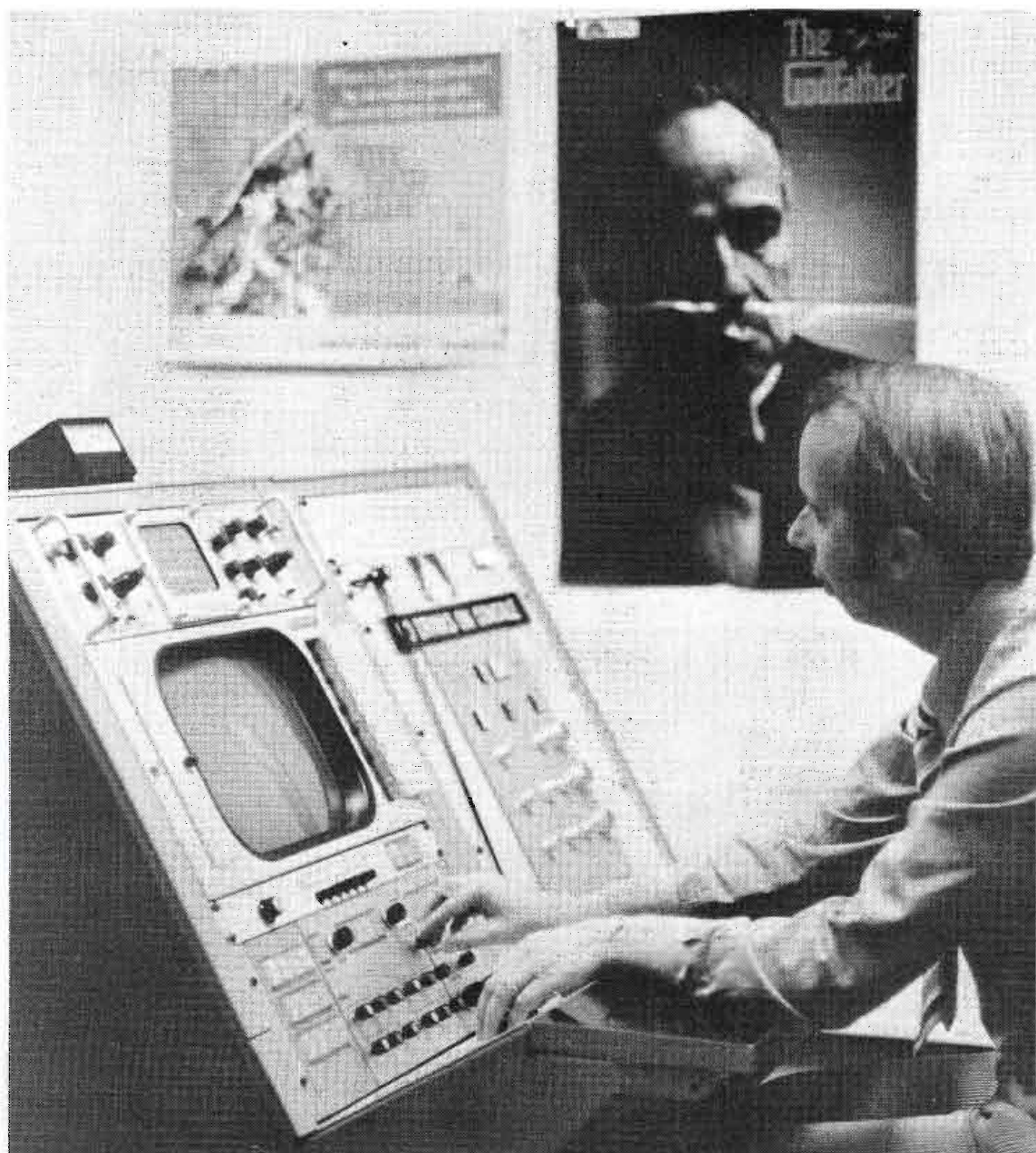
An important part of Vidtronics' capability is a special film-to-tape transfer system. Director of operations Tom Mann is shown using the system. "Godfather" and "My Fair Lady" are recent transfers Vidtronics has done for television.
